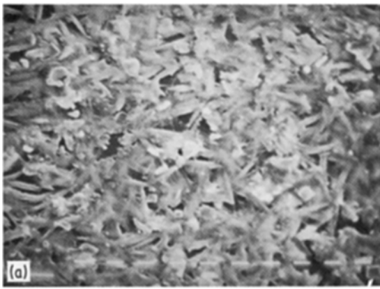
Figure 6 SEM micrographs of \text{Bi}_2\text{S}_3 films prepared by the dip-dry method: (a) 5 dips, thickness 60 nm; (b) 25 dips, thickness 300 nm. Marker size 1 \mu\text{m} .
